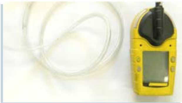
Gas monitor equipped with pump and suction tubing
